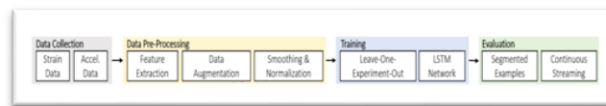
Fig 4.2 Pipeline Process to create a neural network that can classify segmented examples or streaming real-time data
