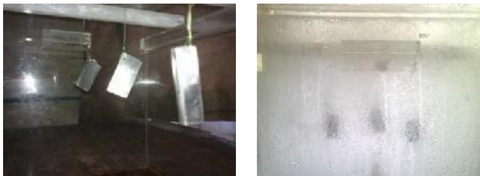
Fig.1 Prepared specimens hanged in the chamber before and after fog
