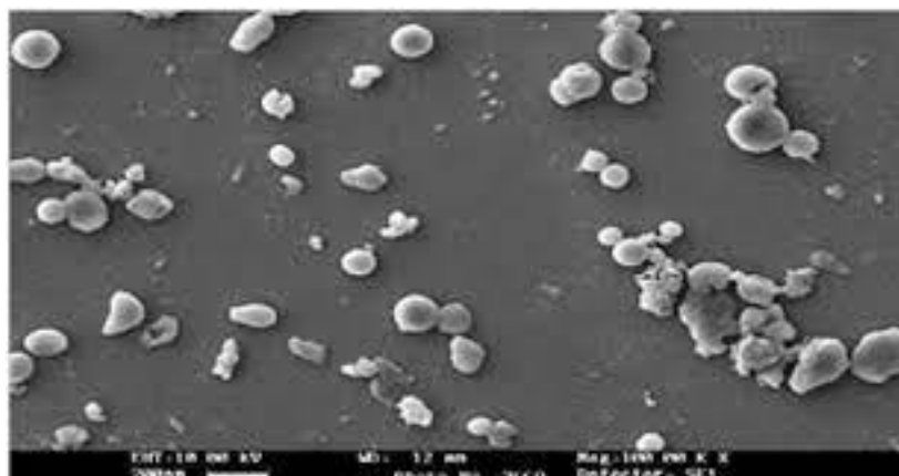
Figure 6: Sem Microphotograph of Layer, Showing Development of Pores
